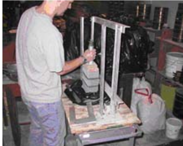
Figure 2 Prism Fabrication Applying Drop Hammer to Consolidate the Mortar Joint
