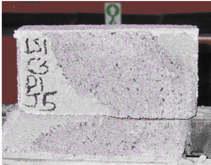
Figure 4 Brick Pull-away Failure (Prism 1, C3-LS1, Joint 5)
