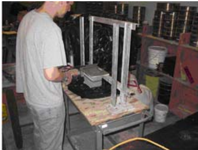
Figure 1 Prism Fabrication Using Jig and Mortar Form
